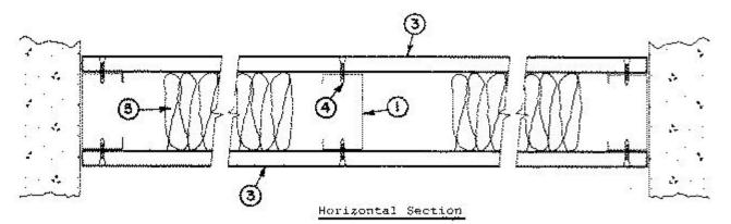
1. **Studs** — Channel-shaped, min 3-5/8 in. wide with 1-1/4 in. flanges and 3/8 in. lips. Fabricated from No. 25 MSG galv steel. Max stud spacing is 24 in. OC. Stud length cut 3/4 in. less than assembly height.
